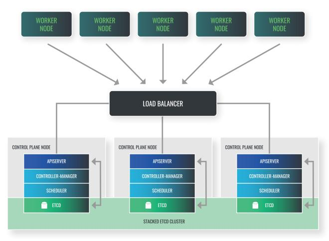
Each control plane has access to individual worker nodes to ensure no single point of failure in your cluster. Placing multiple replicas on separate infrastructure is recommended to remove another single point of failure at the hardware level.
